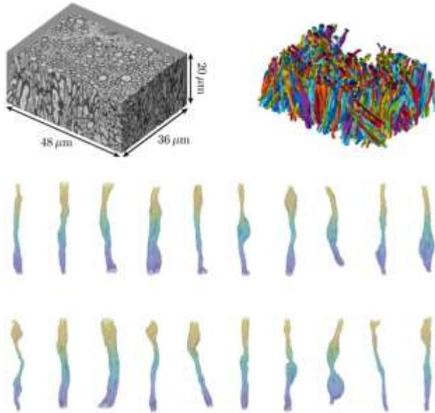
**Figure 2.** Realistic microstructure of the intra-axonal space reconstructed from 3d scanning electron microscopy images of mouse brain genu of corpus callosum.
