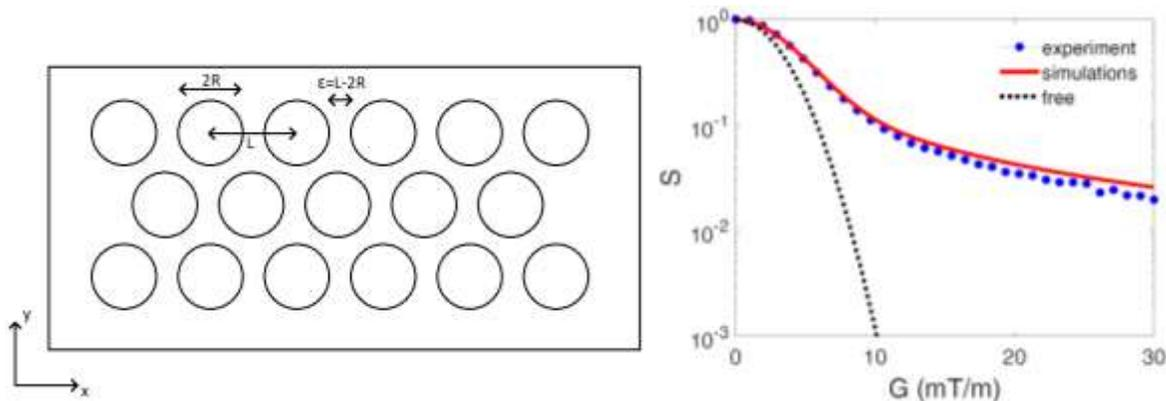
**Figure 1.** (left) Schematic representation of the setup (view from above). (right) Experimental signal (dots) and numerical simulation (full line) show very good agreement. The localization regime signal decays very slowly compared to the signal from free diffusion (dashed line), and significant deviations can be observed at gradients as small as 10mT/m.
